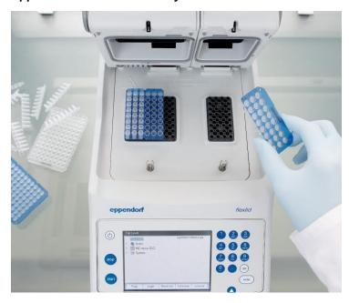
This instrument is said to be ideal for researchers looking to carry out two runs of PCR simultaneously, without any compromise on the number of samples.
