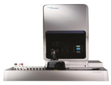
Sysmex Corporation has launched a Sysmex XN series hematology analyzer. The new Sysmex XN series is equipped with a White Precursor Cell (WPC) channel to differentiate abnormal lymphocytes and blasts by using the optical detection system and Fluoroscence flowcytometry. The products are marketed in India, exclusively by Transasia Bio-Medicals.
