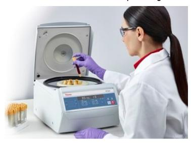
Thermo Fisher Scientific has introduced Medifuge, a small benchtop centrifuge. The new benchtop centrifuge features a unique 2-in-1 hybrid rotor that has interchangeable fixed-angle and swinging buckets to facilitate quick and convenient switching between applications.
