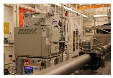
Researchers at the European Molecular Biology Laboratory (EMBL) in Hamburg, Germany, have incorporated a multidetector array size exclusion chromatography (SEC) system from Malvern Instruments (Viscotek TDA -Triple Detector Array) at the laboratory's powerful small angle X-ray scattering (SAXS) beamline to improve the productivity and quality of detailed protein characterization work.
