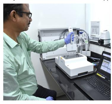
Eppendorf India has added a new capability at Pipette Calibration Facility in Chennai with the installation of 'Speedcal mobile', first-ever installation in India, to calibrate 8-channel or 12-channel micropipettes in less than 30 minutes.
