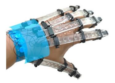
The Department of Physics at the Indian Institute of Science (IISc), Bengaluru has developed a soft, wearable device that exploits the fundamental properties of light to sense a patient's limb or finger movements. The customisable, 3D printed gloves can be remotely controlled, opening up the possibility of teleconsultation by physiotherapists.
