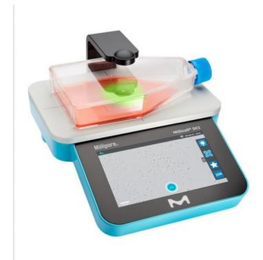
Merck has launched its new Millicell DCI Digital Cell Imager, an instrument that helps improve cell culture lab productivity by assessing a broad range of parameters including confluency, morphology, and cell growth trends, providing faster and more accurate analysis results with reduced user bias.
