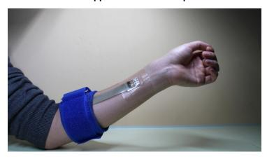
A research team from the Indian Institute of Technology, Bombay (IIT-B) has developed low-cost soft, flexible, and wearable sensors that can be used for diagnosis of pulse rate variability in humans.
