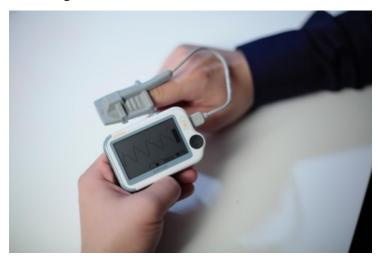
A group of engineers at the Indian Institute of Technology (IIT), Madras, has developed the algorithm for a medical-grade, wearable device called VinCense. The device can be used for unobtrusive monitoring of vital signs including pulse-rate, oxygen saturation, respiratory rate, skin temperature and blood pressure.
