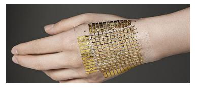
A team of scientists at the University of Colorado, US has developed a new type of malleable, self-healing and fully recyclable electronic skin that has applications ranging from robotics and prosthetic development to better biomedical devices.
